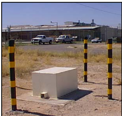
Several monitor wells have been installed at the Park-Euclid WQARF site near locations of historic dry cleaning operations.
