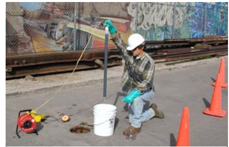
Sampling at the Site from a Monitor Well
